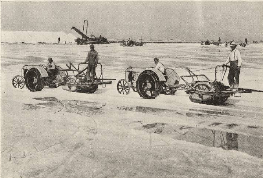
FIG. 4—"Harvesting" solar salt with the aid of machinery at the Morton Salt Company's Burmester, Utah, plant. In the background a portable elevator is piling up a mountain of salt.
