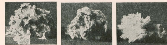
(A) Rags as they appear after leaving the cooker. (B) After passing through the washing process. (C) After bleaching—Just a snowy white mass of clean strong cotton fibres without even a speck to mar their purity.
