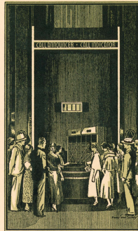
Exhibit 2A. Receiving Dialed Calls at Non-dial Switchboard
