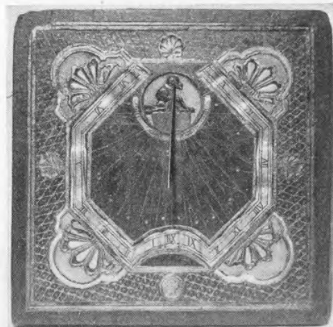
FIG. 43. A.M. 277. HORIZONTAL DIAL FROM INDIA.
