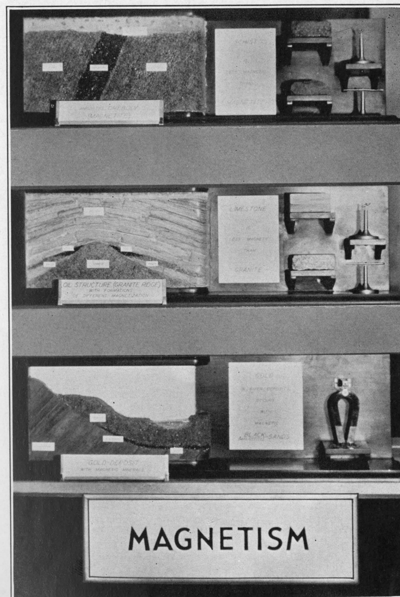
Fig. 4—Exhibits demonstrating rock magnetism. Top—Compass needles show that schist is less magnetic than magnetite. Middle—Compass needles show that limestone is less magnetic than granite. Bottom—Illustrating that gold in river deposits occurs with magnetite.
