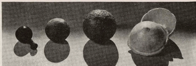
Four Stages in construction of a U. S. Golf Ball
