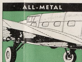
ALL-METAL The 74 ft. wing can support a load of 36½ tons, and the landing gear 32 tons—5 times the plane's weight.
