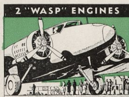
2 "WASP" ENGINES Fully loaded, the plane can fly, if necessary, on only one of its two 550 h. p. supercharged "Wasp" engines.
