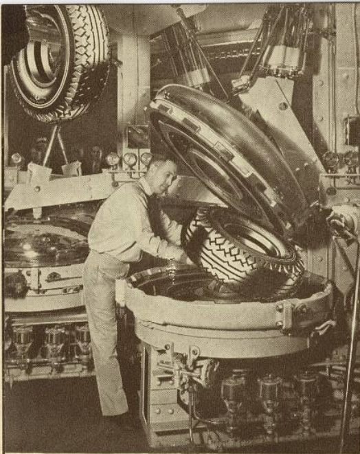
Vulcanizing tire in automatic mold
