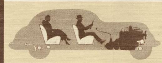
Both front and rear passengers are cradled between the axles in the new Hupmobile, because the engine has been moved forward over the front axle for greater body room and improved balance. There is no pitching for rear seat occupants.
