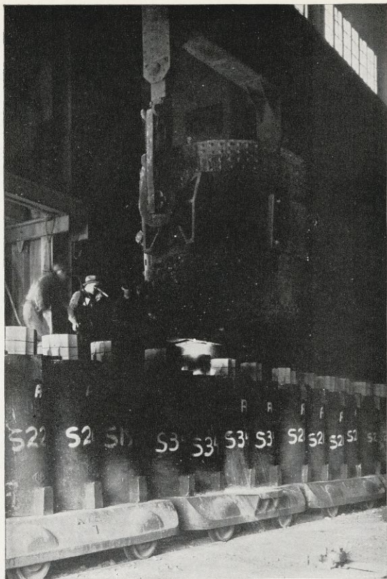
Casting ingots of Timken Alloy Steel in Gathmann-type fluted ingot moulds, hot topped. This is an extra precaution taken by Timken to assure high and uniform quality. The miniature ingots poured in the exhibit in the Chrysler Building are of the same shape, but the actual ingots weigh 5,000 pounds.
