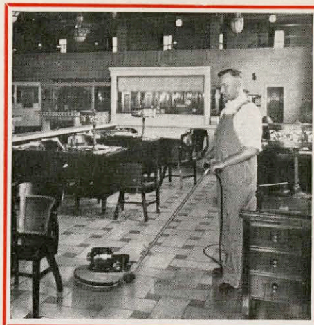
The Hild safety switch (developed in 1929) makes the Hild guaranteed floor machine foolproof. Stops machine instantly when operator releases hold on handle.
