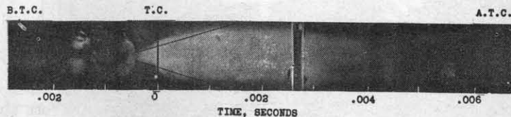
SPRAY PENETRATION AND COMBUSTION WITHOUT DETONATION. INJECTION-ADVANCE ANGLE 30°
